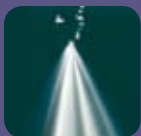
CLOGGED FUEL INJECTOR
