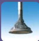
DIRTY INTAKE VALVE
