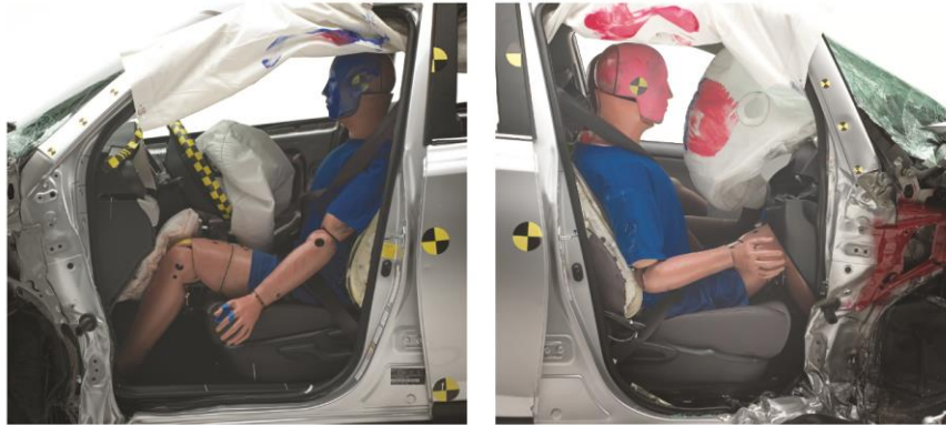
The structure of the Toyota RAV4 held up well in the driver-side small overlap test (left). In contrast, intrusion was severe in the passenger-side crash.
