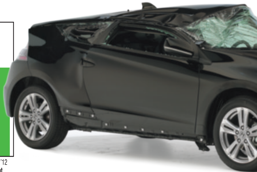
IMPROVED ROLLOVER PROTECTION RATINGS FOR HONDA MODELS, BASED ON TEST OF ROOF STRENGTH-TO-WEIGHT RATIO
