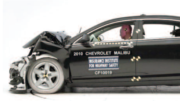
This is a car after a 35 mph full-width crash into a Wabash trailer with a strong guard. The occupant compartment is intact.
