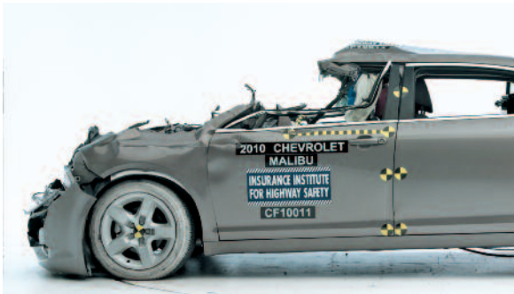
This is how a car looks after a 35 mph full-width crash into the rear of a Hyundai trailer with a weak underride guard.
