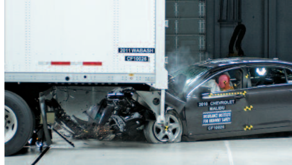
SEVERE UNDERRIDE was the result of this 35 mph, 50 percent overlap crash test with a Vanguard trailer. NO UNDERRIDE resulted when the car struck the back of the Wabash trailer in the same overlap test at 35 mph.
